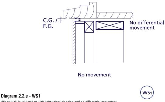
Window cill level junction with lightweight cladding and no differential movement.
