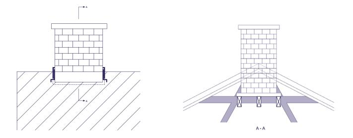
**Diagram - 2.11.d** Alternative support of lightweight chimney on truss roof.
