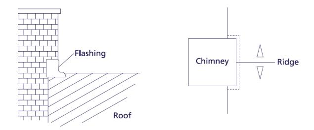
**Diagram 2.3.d** Verge detail with masonry chimney interface.
