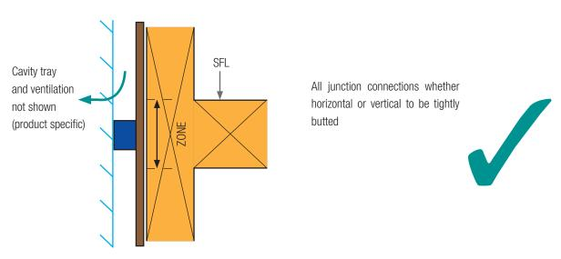
Fig 3b. Cavity barrier correctly positioned against solid timber (cross section view)
