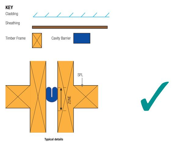
Fig 3a. Cavity barrier correctly positioned (cross section view)
