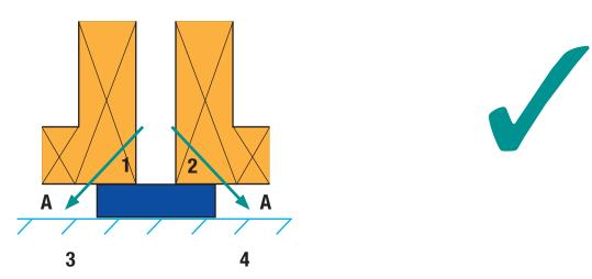
Fig 3d. Party wall to external wall junction - alternative detail (plan view)
