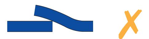
Fig 2b. Cavity barrier incorrectly fixed with gaps
