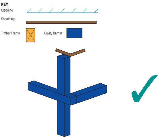
Fig 4a. Corner connection detail - (isometric view)
