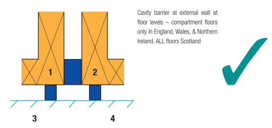
Fig 3c. Party wall to external wall junction-plan (plan view)
