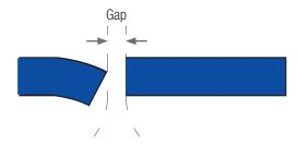
Fig 2e. Cavity barrier incorrectly fixed with gaps
