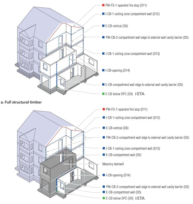
b. Structural timber with concrete/masonry common areas Figure 4.4: Internal frame compartment wall between dwellings and common areas that include a cavity
