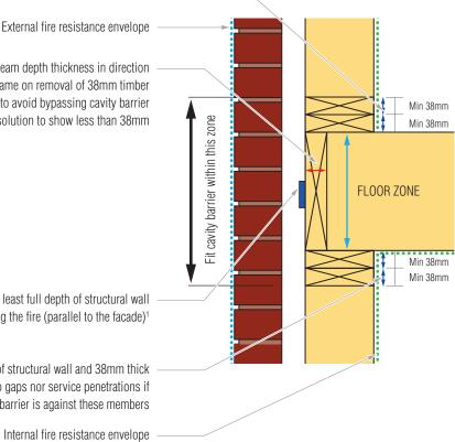
If cavity barrier is within this zone min 38mm timber rim beam depth thickness in direction parallel to depth of structural wall + structural stability of frame on removal of 38mm timber plus service penetrations fire stopped to avoid bypassing cavity barrier or tested solution to show less than 38mm
