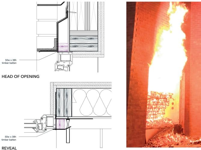
Figure A7.3: Horizontal and vertical fire test for timber batten within the BS8414 test which is a full fire condition of fire from a compartment emitting out of a window
