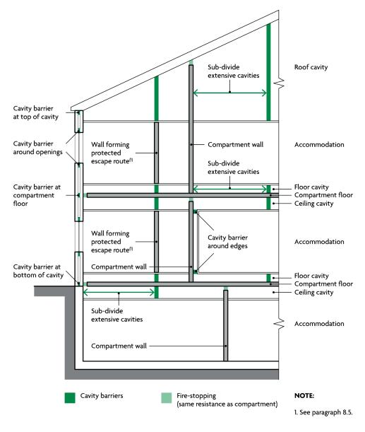
The differences between cavity barriers and fire stopping (download **HERE**)
