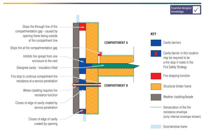
Figure 1.4: Diagrammatic plan of wall assembly - cavity barrier and fire stopping notes regarding function
