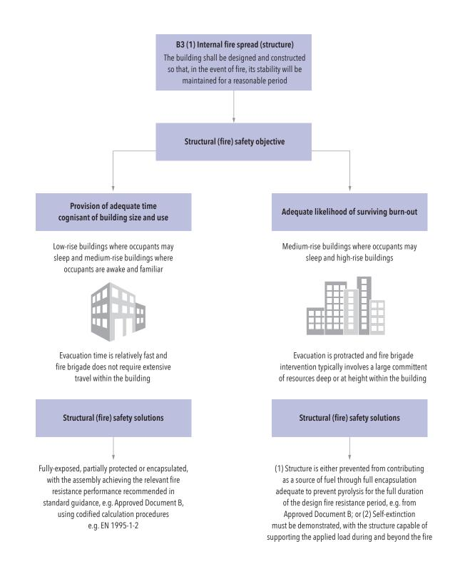
Figure 3: Illustration of the relationship between structural fire safety objectives, compliance routes and design solutions
